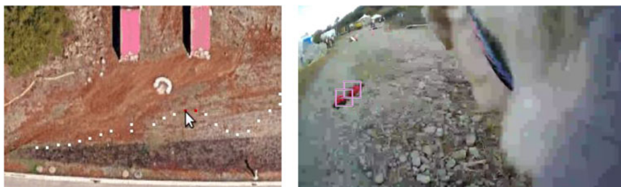
FIGURE 12 Example result generated with backtrack recognition on a live stream from the suit. The dog's path is plotted in dots on the map in the left window, with the red dots indicating high confidence. Placing the cursor near a dot brings up the corresponding frame, shown here on the right. In this result, the system correctly identified the location from which the target (a pair of gloves) was visible. The SAR dog is visible on the right side of the camera image [Color figure can be viewed at wileyonlinelibrary.com ]
