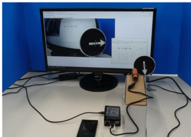
FIGURE 10 Delay measurement set-up [Color figure can be viewed at wileyonlinelibrary.com ]
