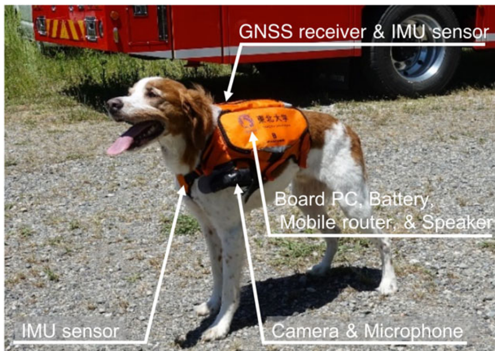
FIGURE 2 Placement of sensors and other system elements in the cyber-enhanced canine suit. GNSS: Global Navigation Satellite System; IMU: inertial measurement unit; PC: personal computer [Color figure can be viewed at wileyonlinelibrary.com ]
